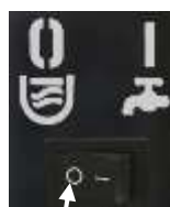
Place switch into position "0" when operating machine with water tank
